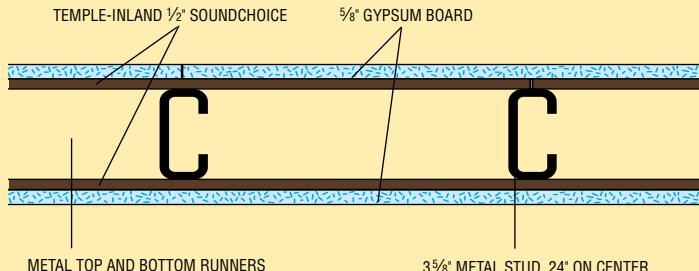
**Warning:** Temple-Inland SoundChoice may smolder if ignited. Do not expose to open flame. Do not expose to prolonged excessive heat above 212°F without sufficient thermal protection. Like wood and other organic materials, SoundChoice can give off toxic smoke if ignited.
