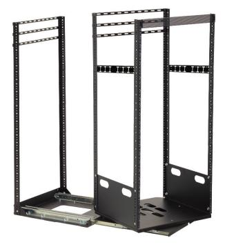
To ensure adequate cable length at the rack's maximum turn radius, rotate the rack fully before tying cables to rear lacing panels (see pg. 3).
