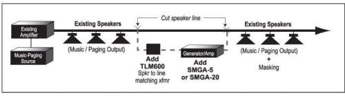
Typical masking addition to an existing system using a line matching transformer and masking generator amplifier connected to the speaker line.
